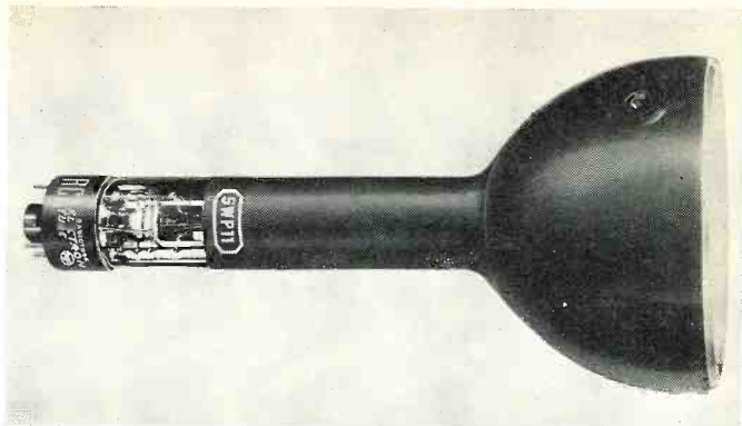
Fig. 4. RCA's 5WP11 transcriber kinescope for TV film work.
