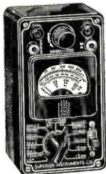
Model 770 is an accurate pocket-size V.O.M. Measures only 3 1/8" x 5 1/2" x 2 1/4".
